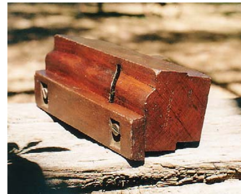
Underview of plane showing detail of Adjustable fence.
