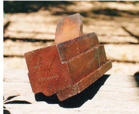
Front Corner of the plane. Note the broad double gouge cut at the end of the shoulder.
