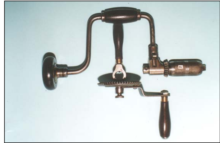
Photo 2. The Millers Falls brace disassembled to show the post and ring attachment. Note the indentation on the post and the locking pin protruding through the ring.
