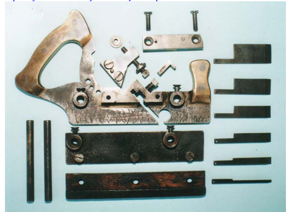
Photo 2. Disassembled layout of the plane. The six blades indicate that the plane was intended for much use.
