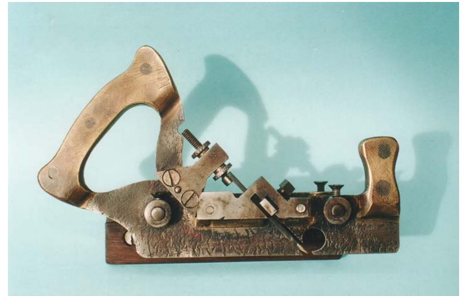
Photo 1. Note the unconventional "blade holder", also the method of attaching the depth adjustment assembly to the body of the plane.
