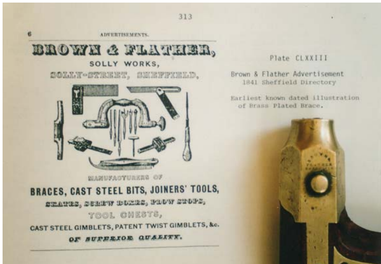
Photo 2. The brace pad photographed against Ken Roberts' reprint of the 1841 advertisement taken from the Sheffield Directory.
