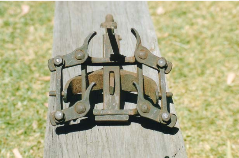
Photo 2: The underside of the J. Woodhead floor cramp. It is evident that all parts are straight off the anvil, not a file mark to be seen. The holes for the pins have been punched through, not drilled. One could confidently conclude that this hand tool was completely hand made.
