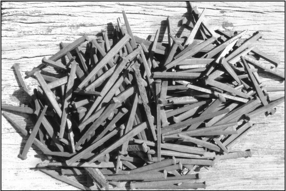
A large handful of shear nails with secondary worked heads, nails 50mm long.
