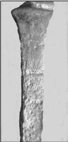
"Grip"marks on the side of a hand-wrought nail made when the nail was held while shaping the head.
