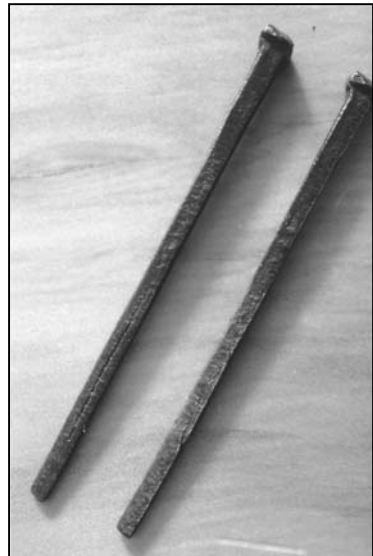
Lamination separation hand-wrought nail
