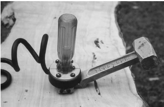
The hammer in position to lever out the electrodes. The line above the base should be aligned with the direction of the grain. Positioned for photograph, not testing.
