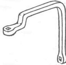
FIG. 6.—A Crank, fastened in a vice, and used to hold beads. Each arm is about 8 inches long.
