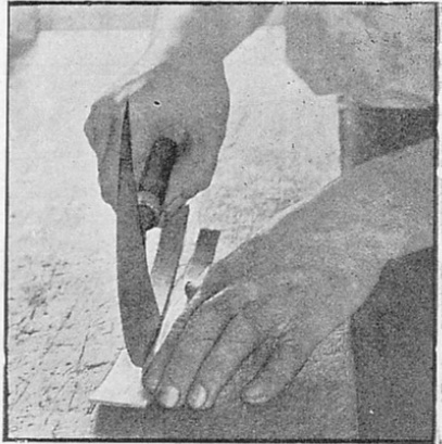
Fig. 8.—Cutting with the Round Knife.
