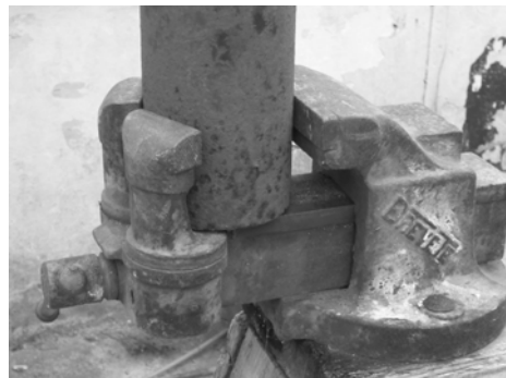
Fig 4. The jaws rotated to hold a large pipe section.
