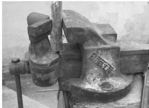
Fig 5. Counter-rotated jaws to hold a smaller pipe
