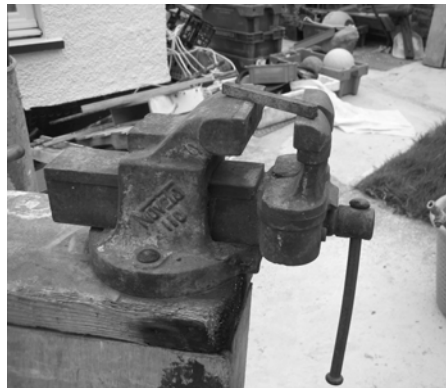
Fig 3. With the square bar removed to allow the jaws to rotate.
