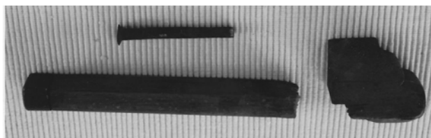
The broken stem and rivet.
