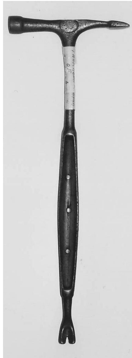
The German slaters hammer, top of the next column, is another interesting example of several tools in one, hammer, hole-punch, nail puller, ripper and dresser. The compound grip would be a good insulator when working in the mid day sun. The roof slater certainly would need to lighten his tool bag when working on a sloping roof, this combination that certainly does that.
