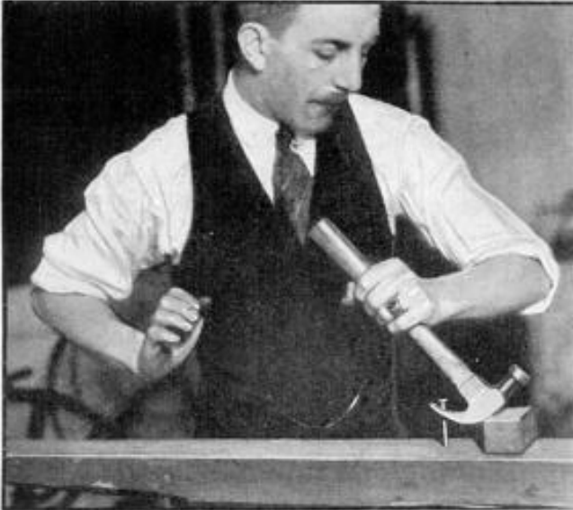
Hitting a hammer handle violently to draw a stubborn nail often snaps the wood in two
