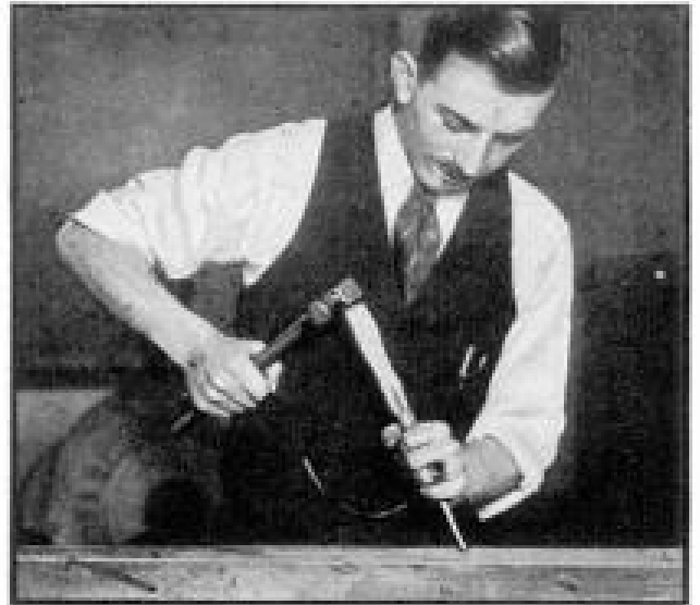
Using the flat side of a hammer to drive a paring chisel generally will ruin the handle
