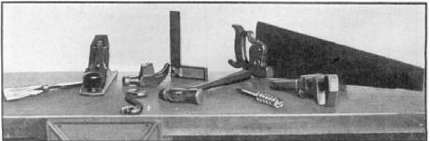
A group of tool casualties. The saw has lost several teeth, the bit has been bent, the try-square misused as a pry, the plane dropped and broken, and other tools damaged by similar abuse
