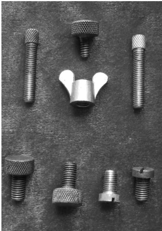
Parts from the Record #050 – parts at top are 55 degree thread form parts at bottom are of 60-degree
