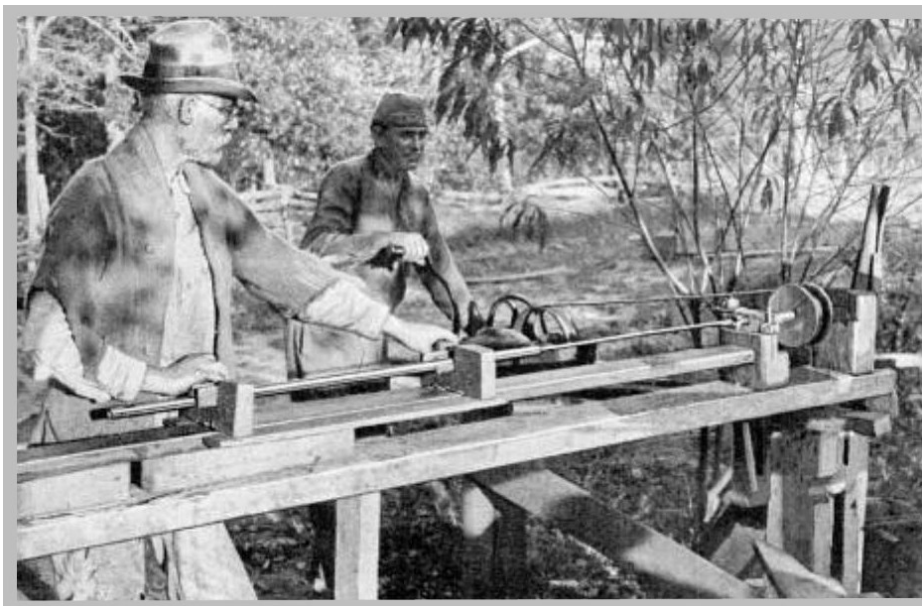
BORING. . . At left, after the barrel has been welded, it must be bored and the delicate task of feeding the bit by hand is done by the master himself, as the value of the gun largely depends upon this operation. The apparatus may appear crude but the guns produced have unbelievable accuracy. Above, No. 1, long bit with hickory guard; No. 2, the short bit, the first used. No. 3 and 4, rifling tools
