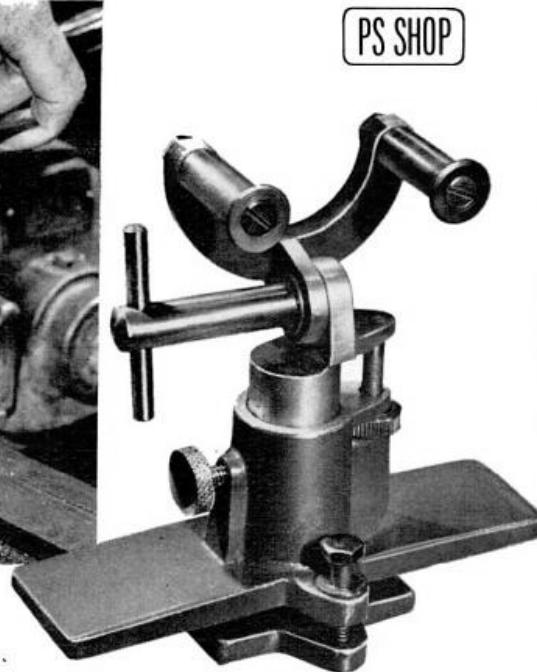
Flanged rollers guide the familiar hand file to new accuracy and usefulness. The device clamps across the lathe ways by means of a shoe underneath. An elevating screw and nut raise or lower the post. The horizontal T bolt loosens the yoke for tilt adjustment to suit the job at hand.
