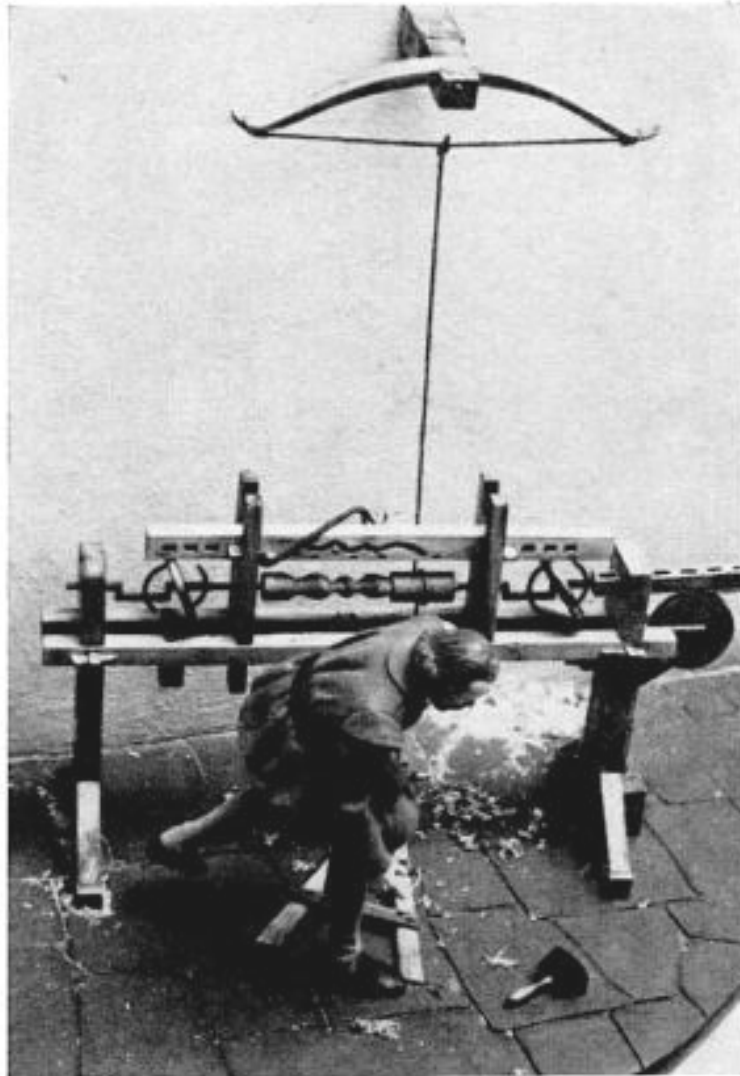
Diorama shows that automation is nothing new. A wood lathe of 1569 used a template-tracing device to speed cutting of irregular shapes.
