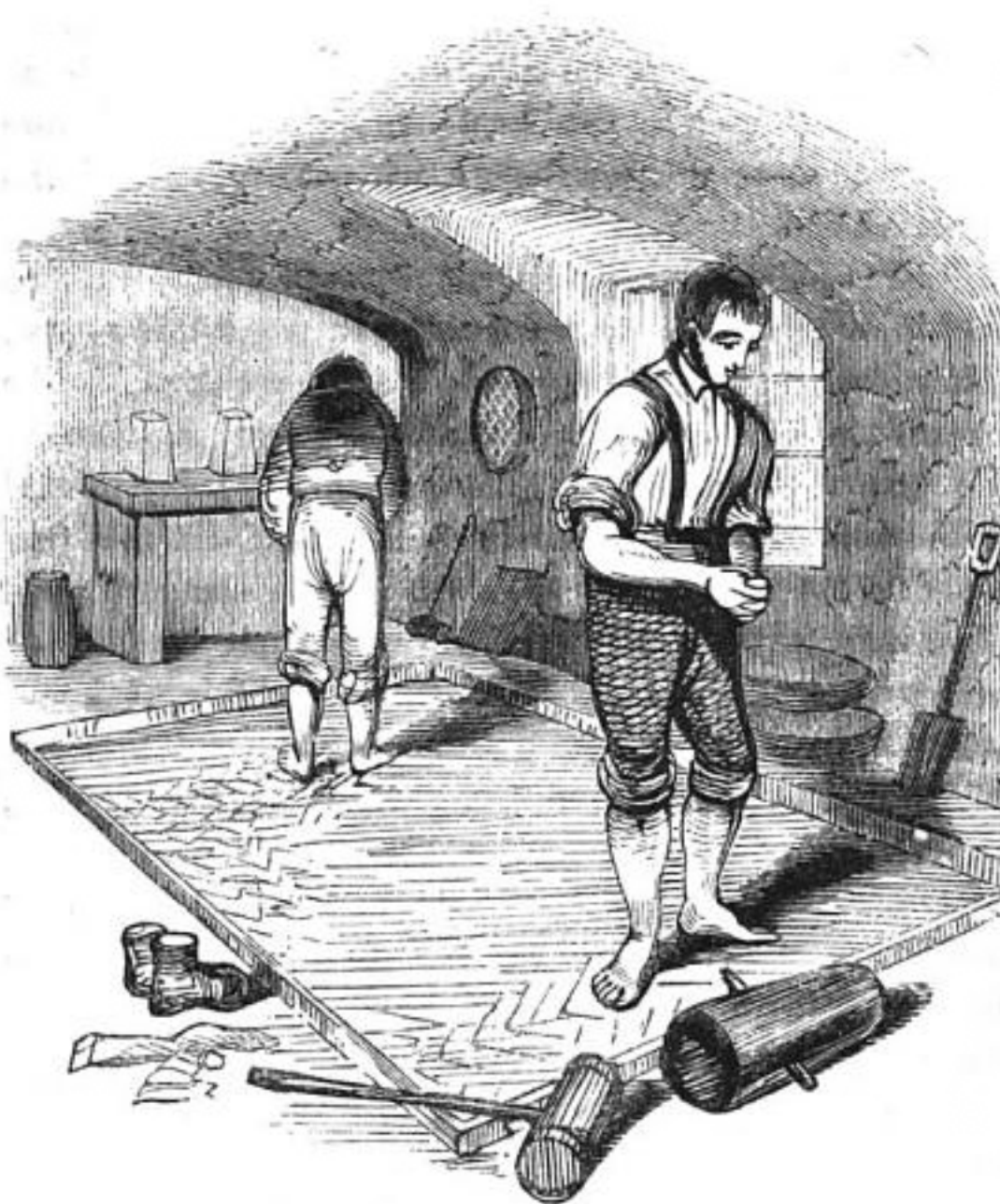
Preparing Clay for Steel-melting Pots.
