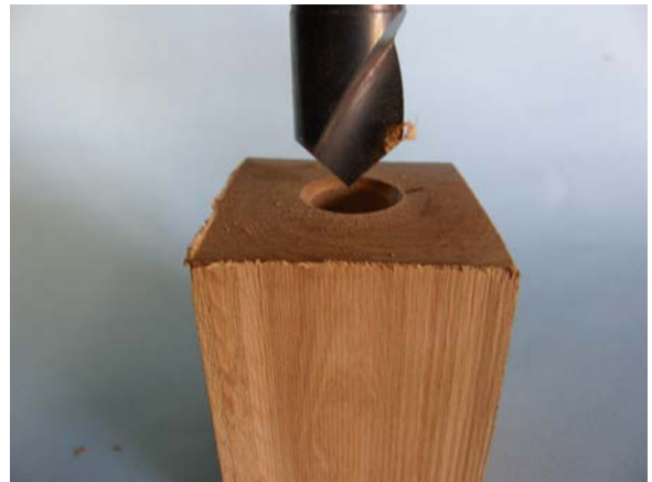
2c Countersinking bottom counterbored hole
