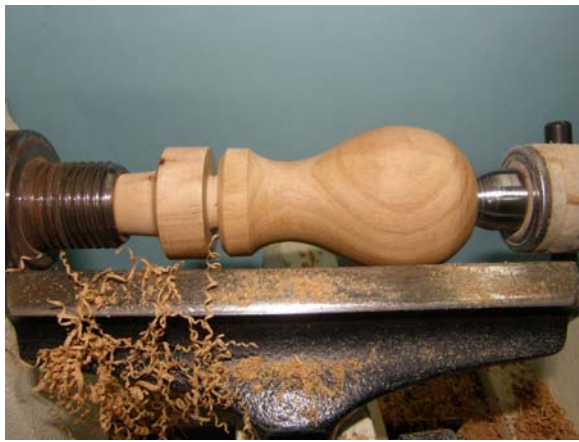
4c Turned to shape ready for sanding
