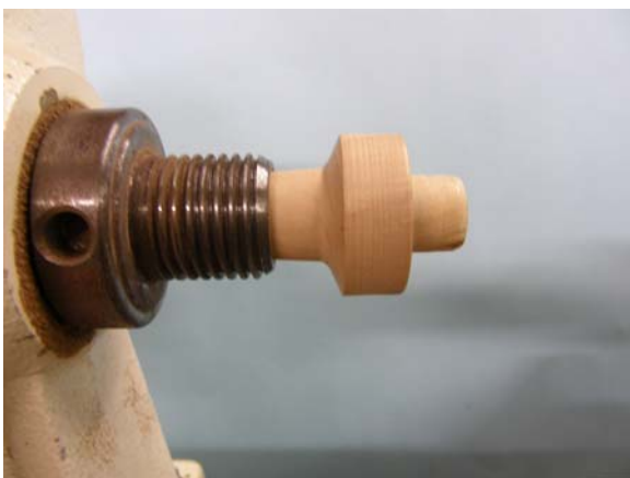
3a. Spigot fitted into mandrel.
