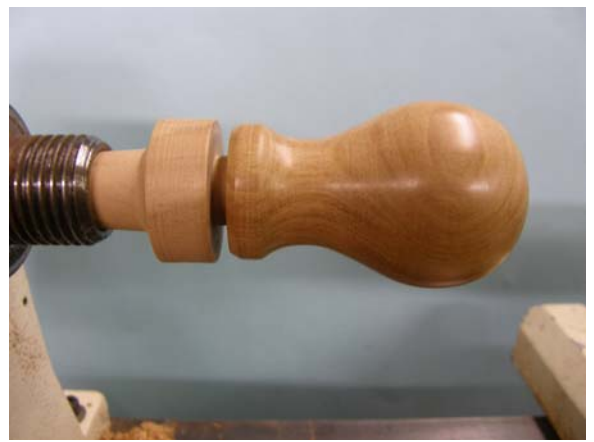
5 Held by spigot for fine sanding and buffing
