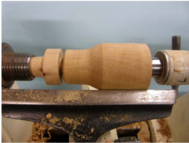
4a Turned down to effective diameters
