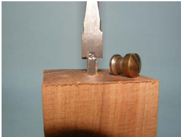
2b. Counterboring using modified spade bit
