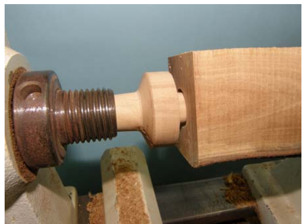
3b. Stock counterbored to fit spigot
