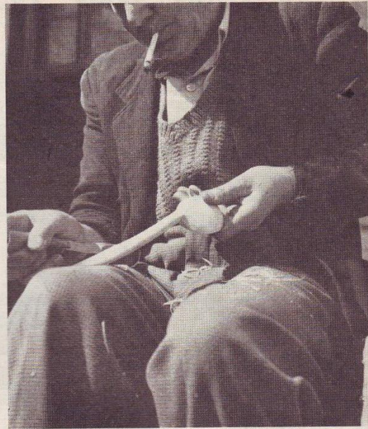
FIG. 4. SMOOTHING THE HANDLE AND BACK OF BOWL WITH SPOKESHAVE
