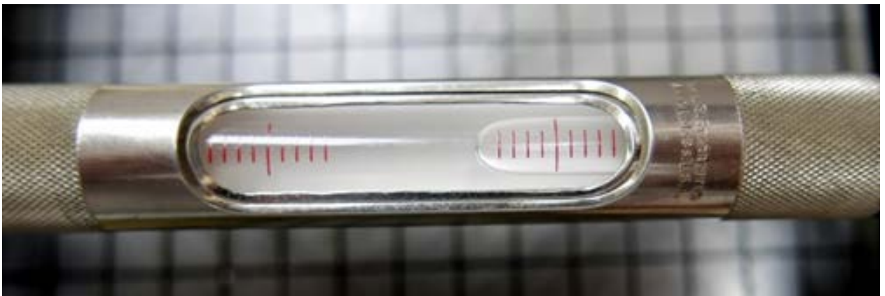
Figure 6 - Starrett 98 New Level Vial Test Fit
