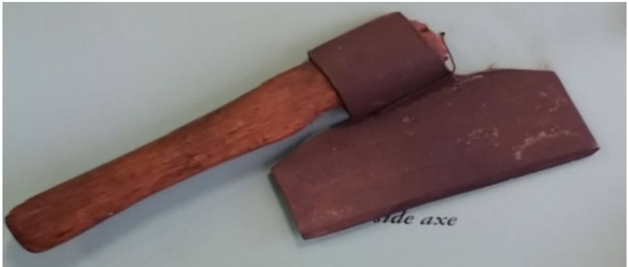
Side Axe Used to shape the staves.
