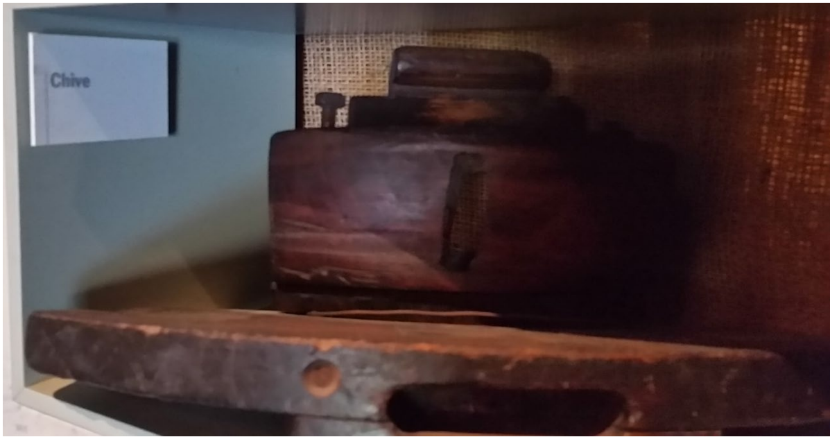
Coopers Chiv Used to give a perfect curve to the inside of the chime ready for the groove to be cut for the head of the cask.
