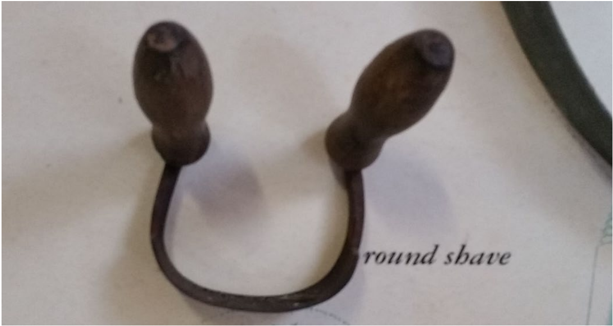
Round Shave Used to smooth the inside of the barrel'
