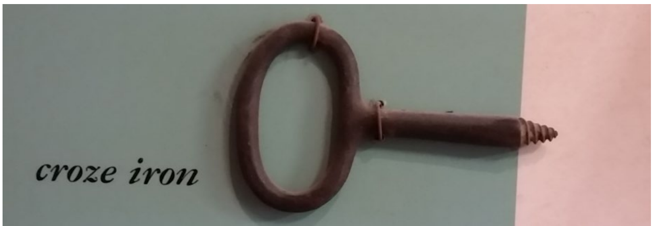
Croze Iron or Vice Used to hold the cask head.
