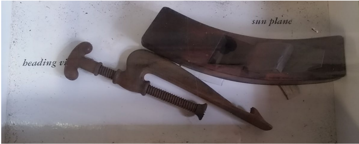
Coopers' Topping or Sun Plane Used to smooth the ends of the barrel.
