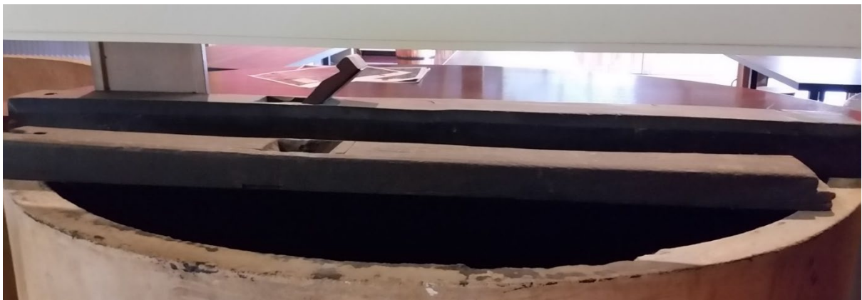
Jointer Planes Used in the inverted position with one end supported on a simple trestle.
