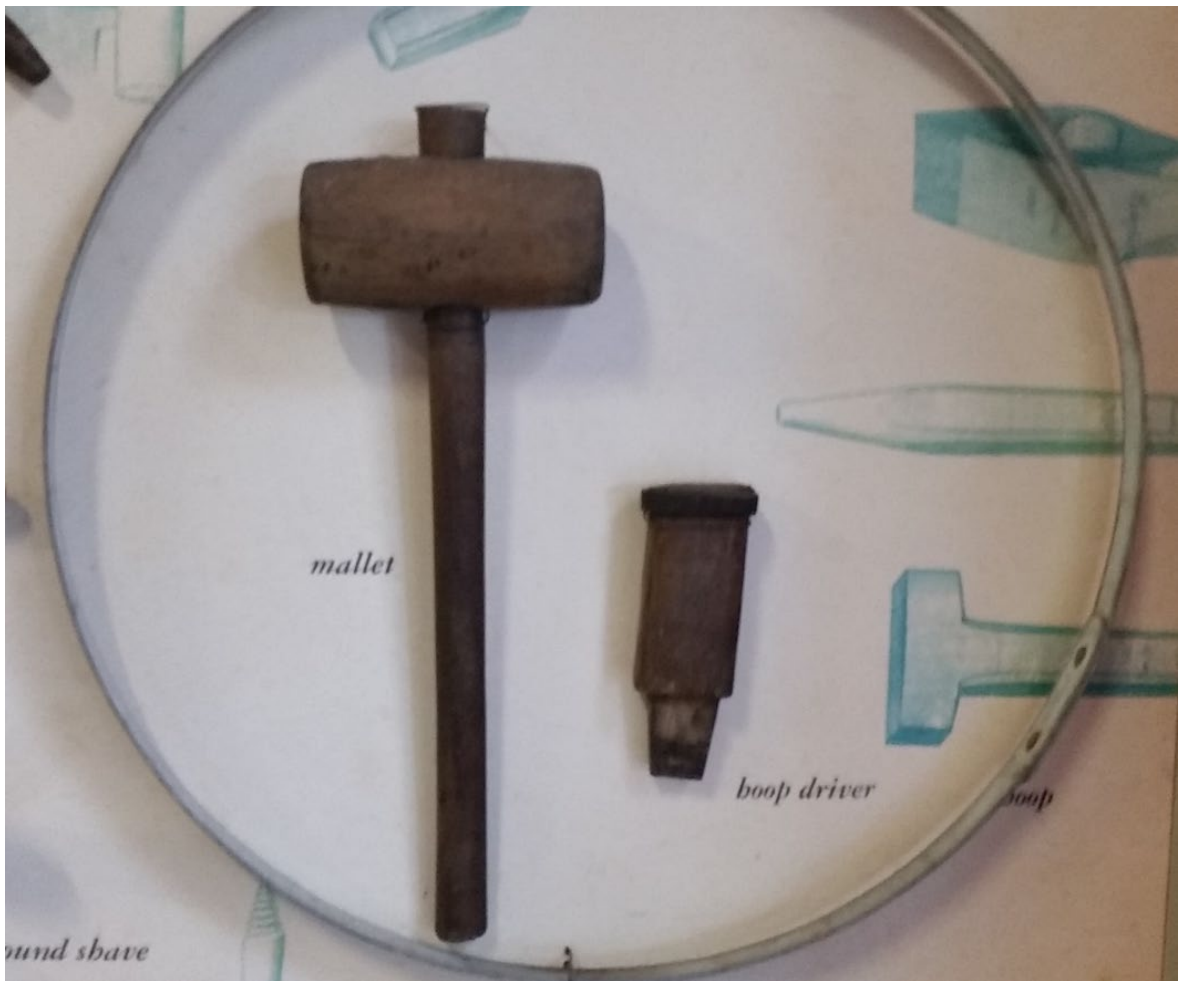
Hoop Driver and Mallet Used to install the barrel hoops.
