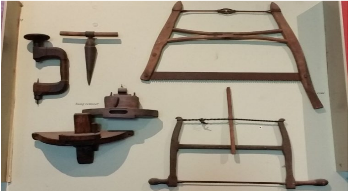
Bow saws Used to cut the head to shape.
