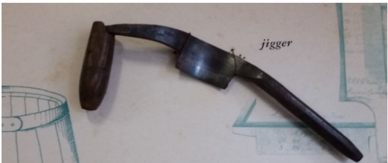
Jigger or Crumb Knife Used to shape the inside of a stave.
