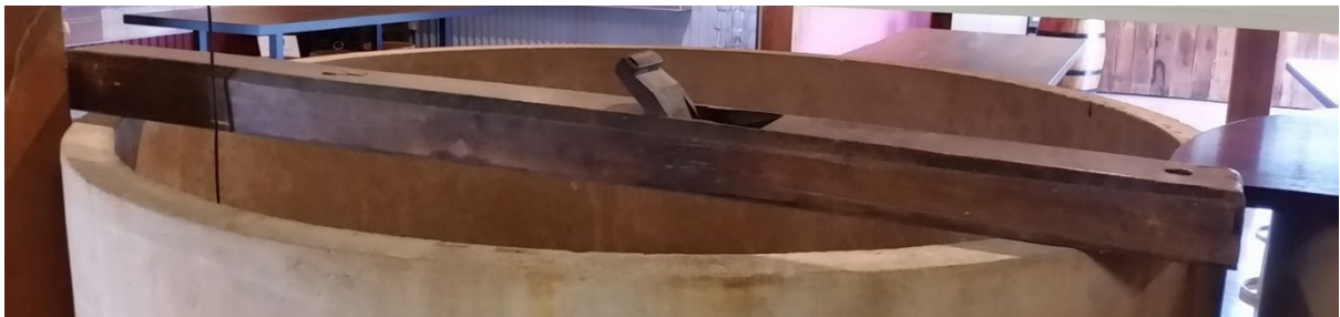
Jointer Plane Off the trestle
