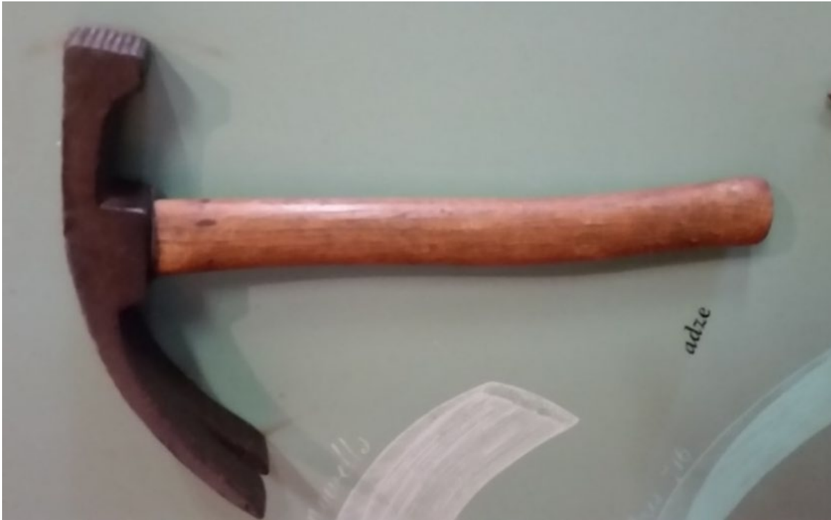
Adze Used to chime the cask
