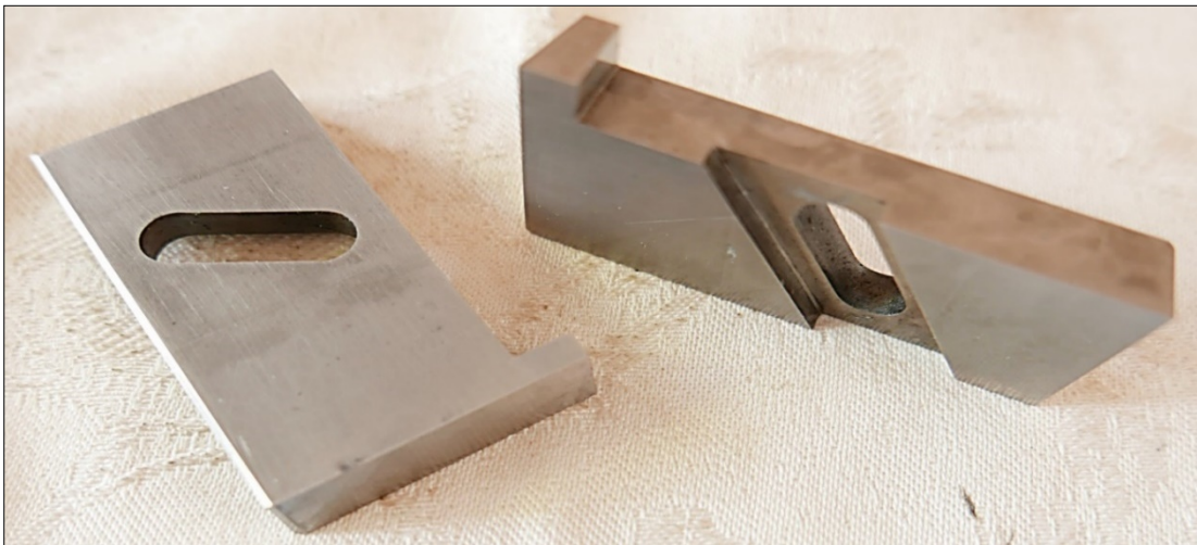
ABOVE: pair of David Brown HSS reamer blades for stepped or blind bores
