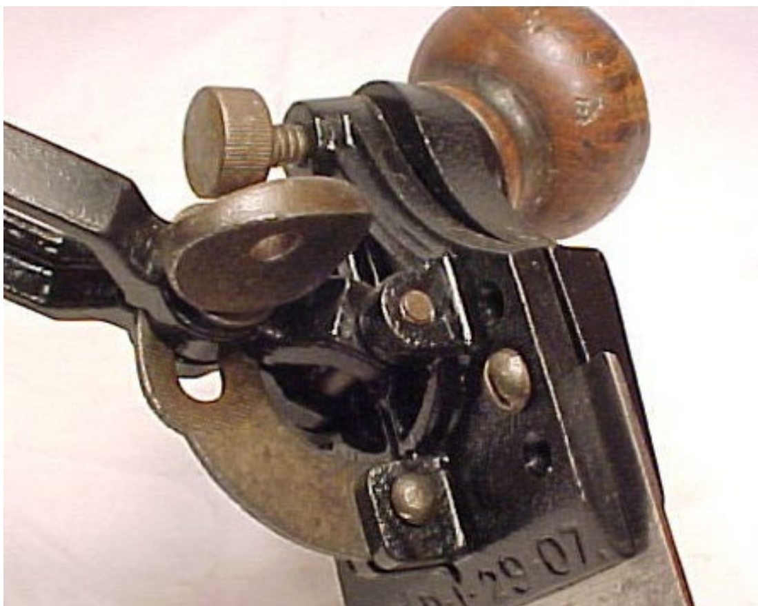
Photo of another No.82 showing the original thumb screw with 'handy' hole
