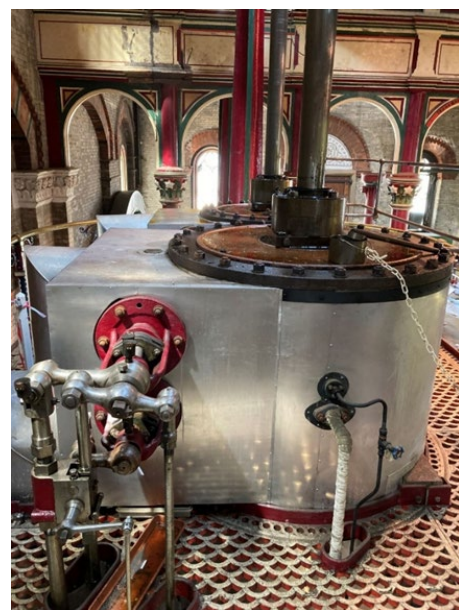
The triple expansion cylinders restored
