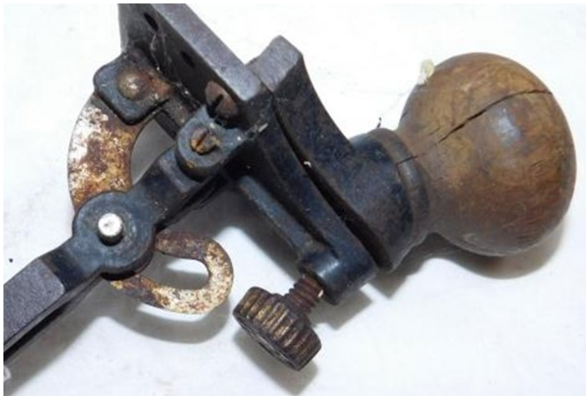
Photo of another No.82 showing the original pivot pin with screw slot.
