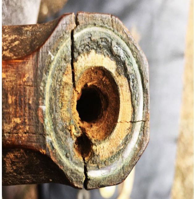
ABOVE: Extensive damage to the head end of the frame
