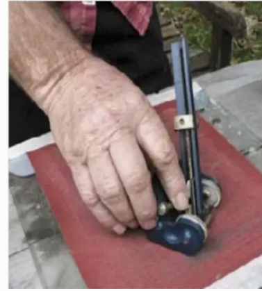
Sharpening a drill bit with the Eclipse 39 jig
