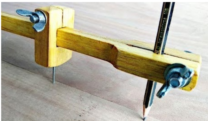
Fig.2. A homemade beam compass.
