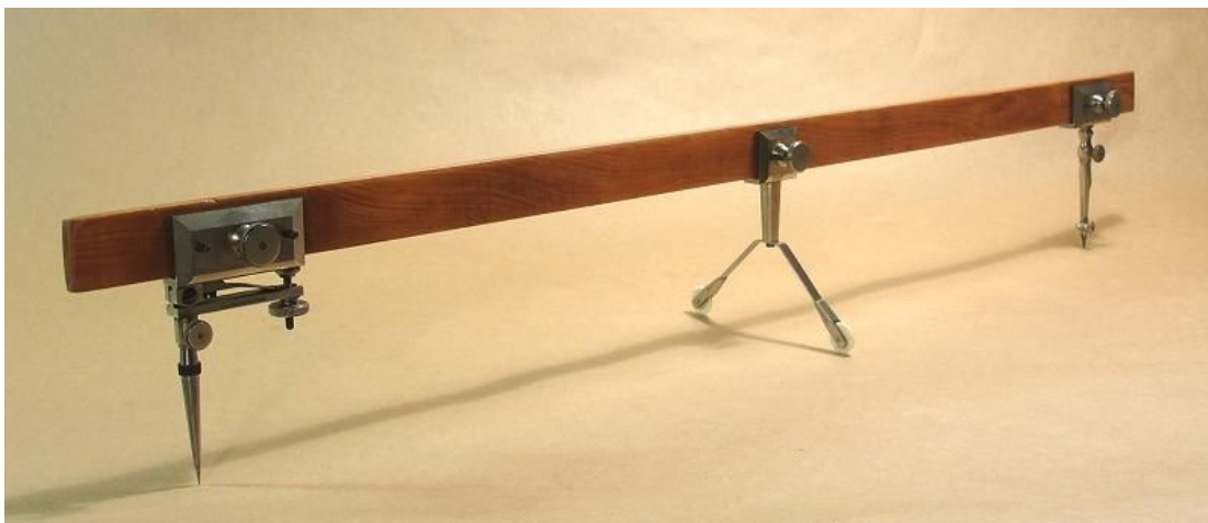
Fig.9. T. Alteneder & Sons, Beam Compass Set. Philadelphia, USA. The set would have been bought in a small case lined with velvet. Circa, Mid-20th Century. A set of wheels for extra stability and accuracy.
