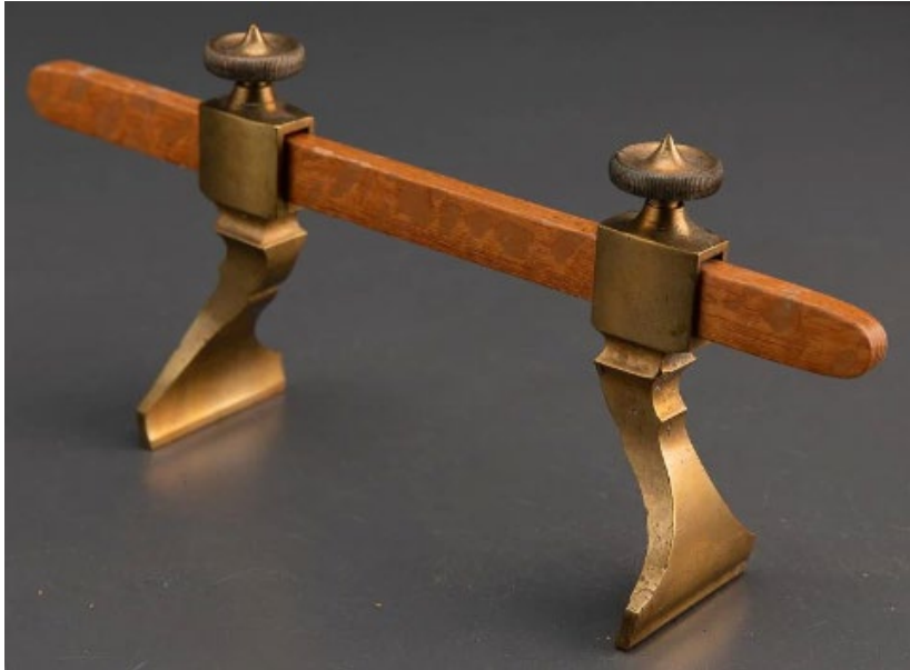
Fig.3. Very Unusual Flat Bladed Trammel Points on a lacewood Beam. The trammels are 4 & 3/8" high.
