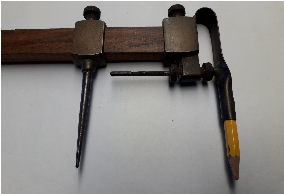
Fig.6. My Beam Compass, unmarked although possibly made by the Stanley Rule & Level Co. Possibly the Henry Haslam patent of June 7, 1892, for the pencil holder attachment. The manufacturer was The Stanley Rule & Level Co. - New Britain, CT and one of the witnesses was Justus A. Traut.
