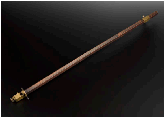
Fig.1. Made in 1775-1795 by George Adams in Fleet Street, London. He traded at Shoe Lane, London (1733-8), Tycho Brahe's Head, Fleet St., London (1738-57) & 60 Fleet St. (1767) succeeded by George Adam the Younger. The beam trammel in Fig.1. Consists of a mahogany beam inlaid with a boxwood scale of 0 - 33 inches and divided into tenths. The pointer can be finely adjusted by means of a micrometer screw one end.
