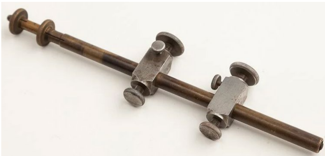
Fig.4. Unusual Telescoping Beam Compass. For drawing larger circles or curvatures larger than those possible with the small compass sets. A scaled beam is required to carry the two
