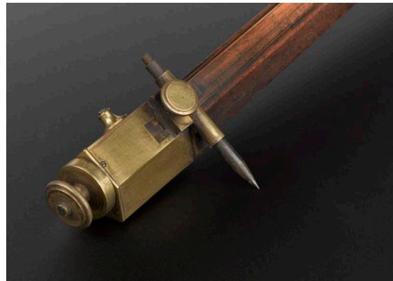
Fig.1. Made in 1775-1795 by George Adams in Fleet Street, London. He traded at Shoe Lane, London (1733-8), Tycho Brahe's Head, Fleet St., London (1738-57) & 60 Fleet St. (1767) succeeded by George Adam the Younger. The beam trammel in Fig.1. Consists of a mahogany beam inlaid with a boxwood scale of 0 - 33 inches and divided into tenths. The pointer can be finely adjusted by means of a micrometer screw one end.
