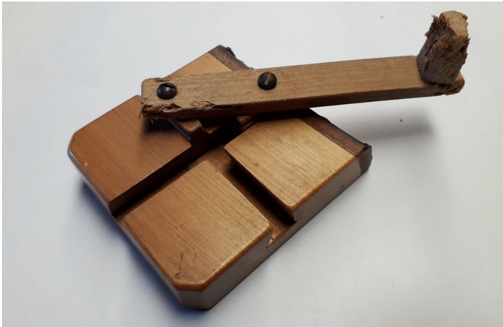
Fig.12. If my Ellipsograph looks like the handle has been chewed by the dog, it does because it has.
