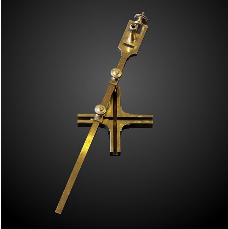
Fig.10. Often referred to as Trammel of Archimedes. An Ellipsograph on display at Musée d'histoire des Sciences de la Ville de Genève. A trammel of Archimedes is a mechanism that generates the shape of an ellipse. It consists of two shuttles which are confined ("trammelled") to perpendicular channels or rails and a rod which is attached to the shuttles by pivots at fixed positions along the rod.
