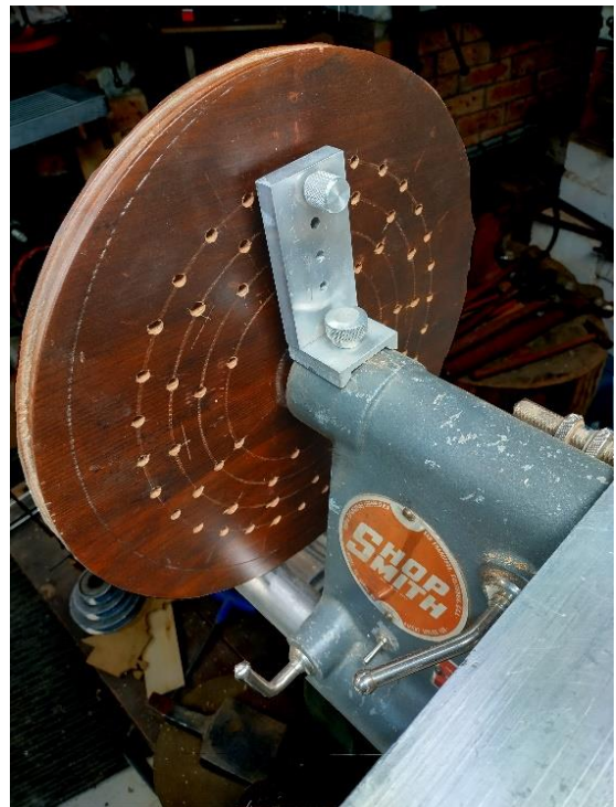
ABOVE: The 15inch slow speed pulley set up for use with the indexing head.
