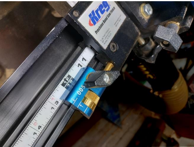
BELOW: The 'Kreg' micro adjuster allows you to rip in 5 thousandths of an inch increments.
