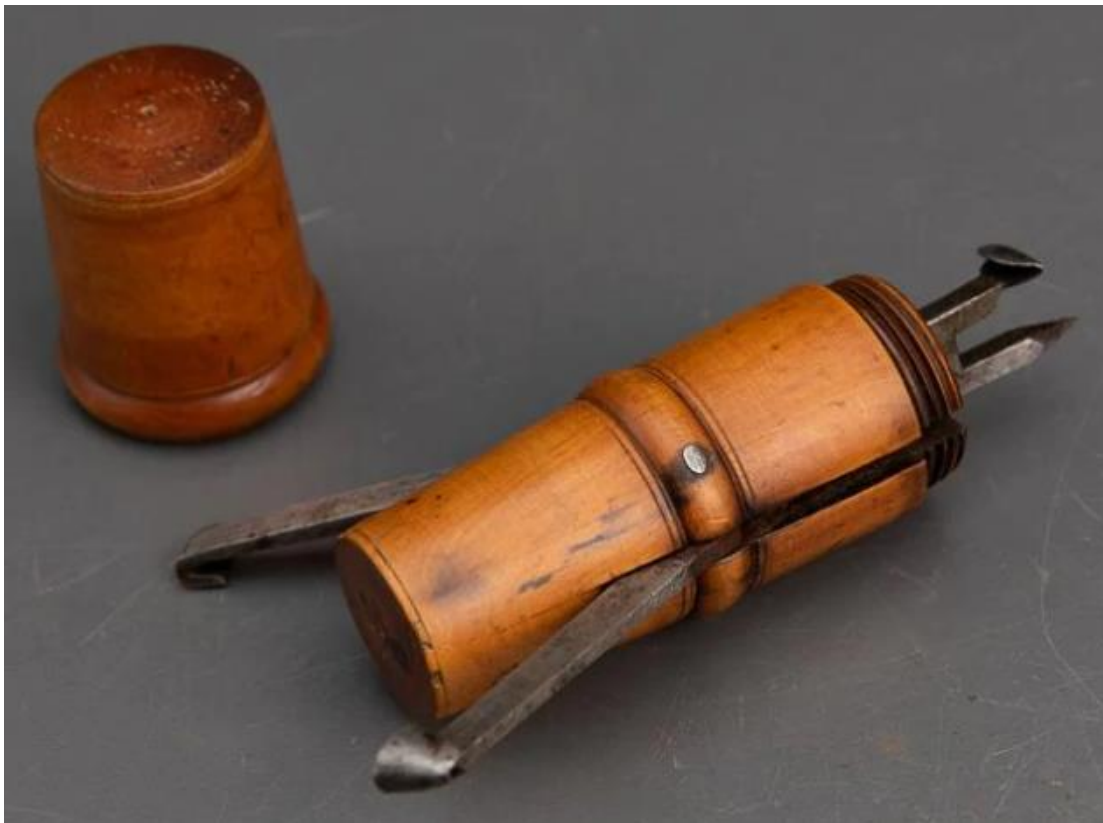
Fig.9. A boxed timber scribe with with three groove-cutting blades.
