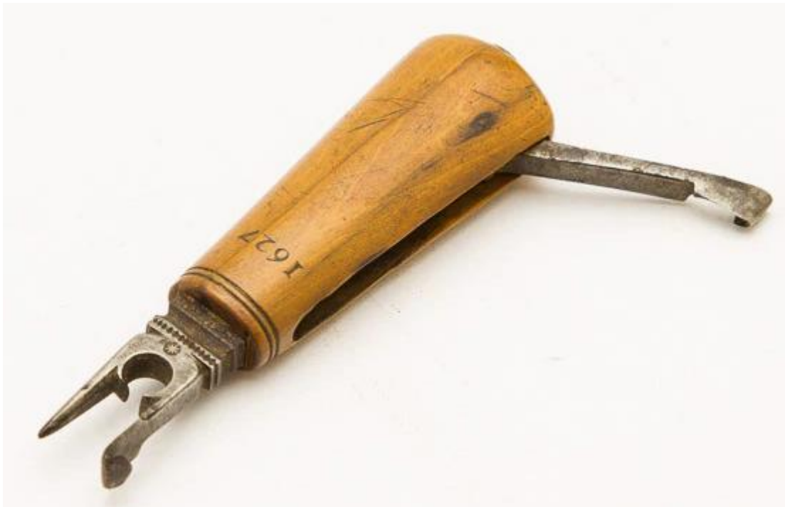
Fig.8. A very early Timber scribe / race knife dated 1627. Most likely Dutch. Many were made using Buffalo Horn, boxwood and Beech.
