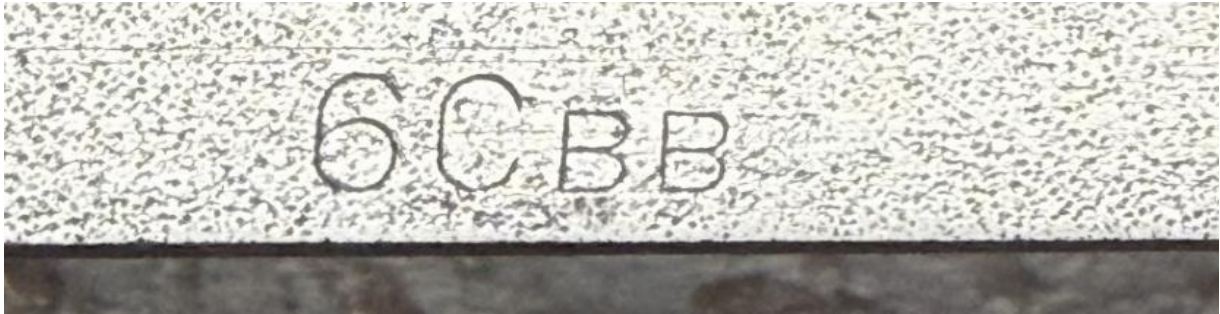
ABOVE: Cheek markings on the 'impulse' buy: - 'C' for Craftsman Millers Falls 'BB'
