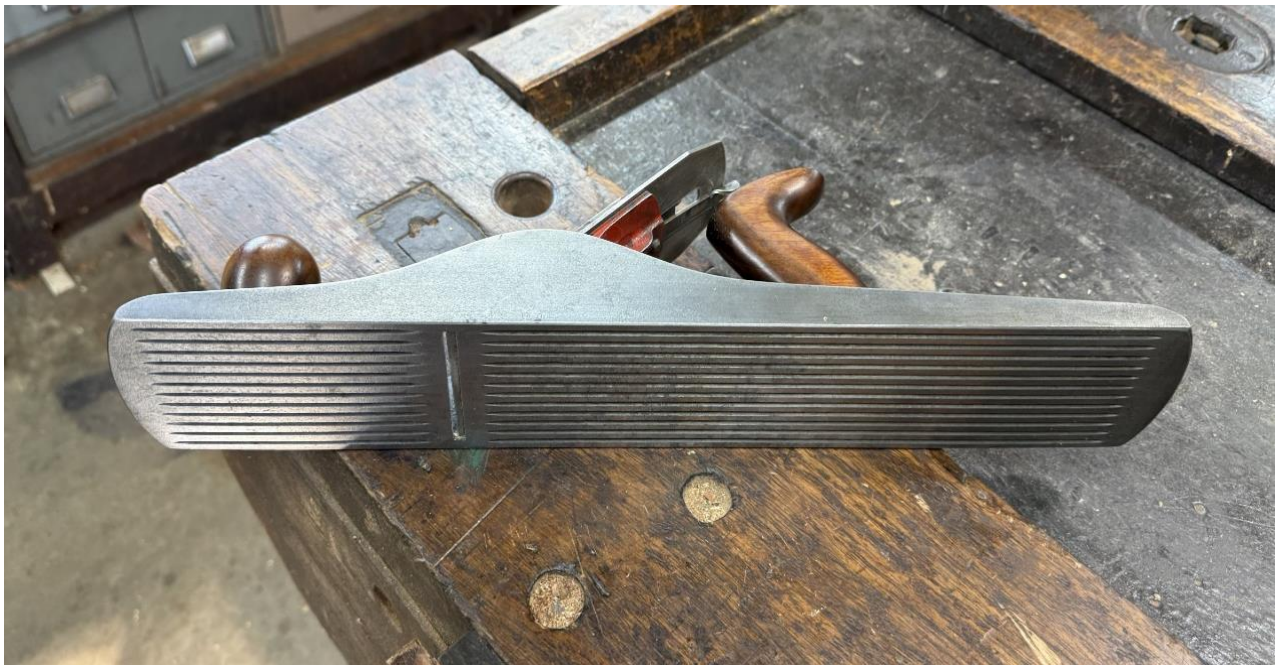
ABOVE: Narrow mouth and no damage to the corrugated sole
