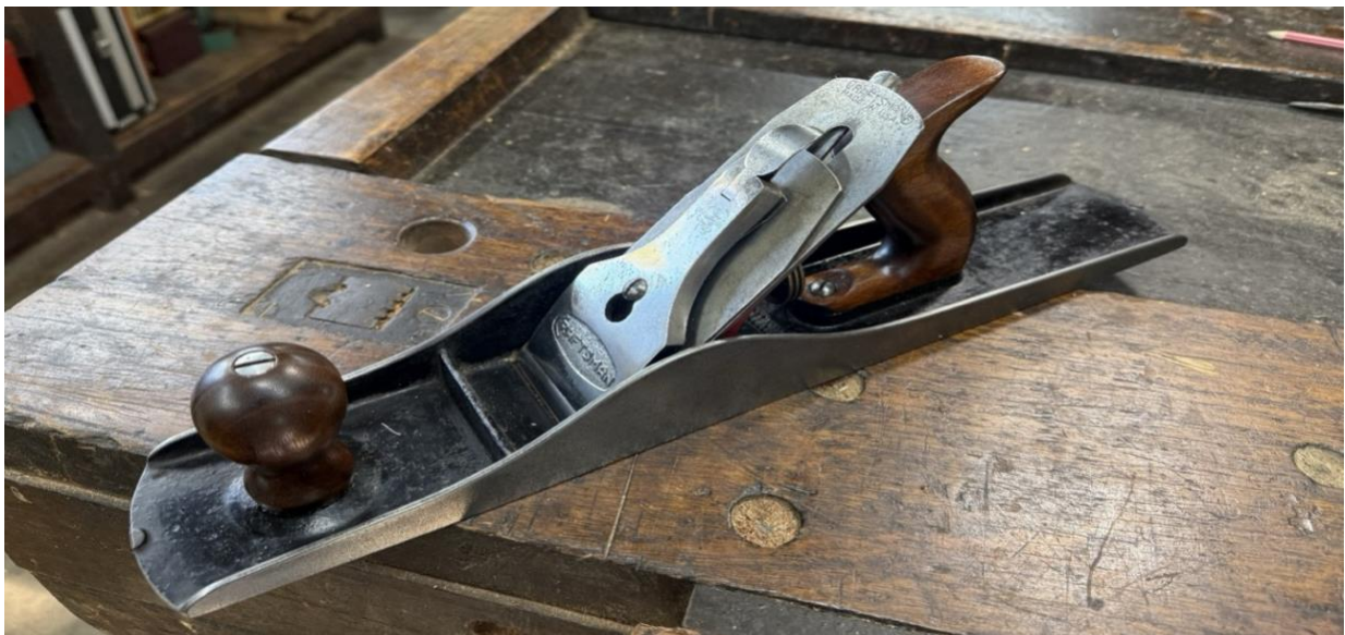
ABOVE: Note the correct seating of front knob and original black Japanning 95% intact
