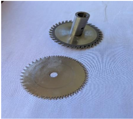
ABOVE: Proxxon 80tpi wood blade with a 36tpi TCT blade on a 10mm arbor - both 85mm dia
