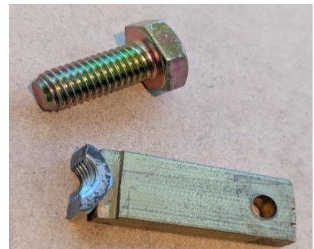
A half M10 nut soldered to brass strip to make thread follower for an M10 bolt
