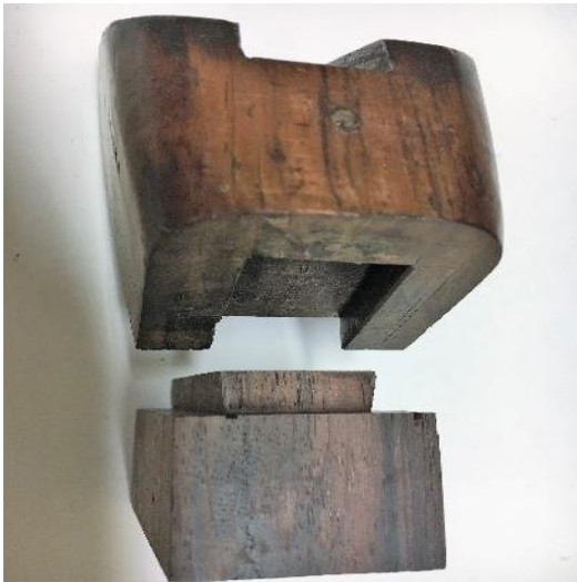
Figure 6: Sliding Dovetail Core attached to Rosewood core.
