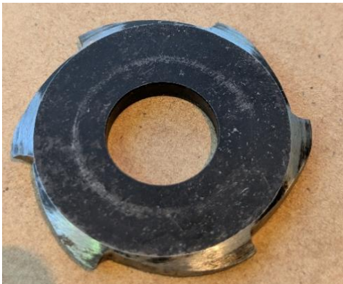
The finished 6-tooth cutter with relief filed between the teeth.
