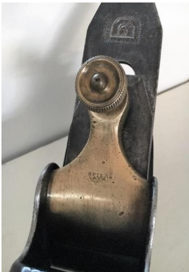
Figure 5: Cleaned gunmetal lever and blade
