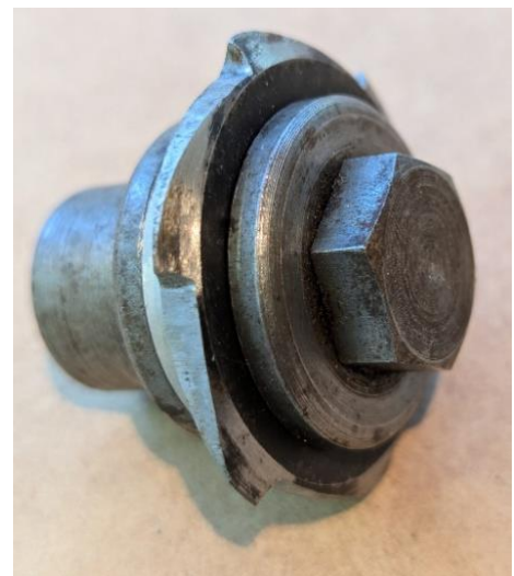
The cutter mounted on the Unimat grinding wheel arbour.
