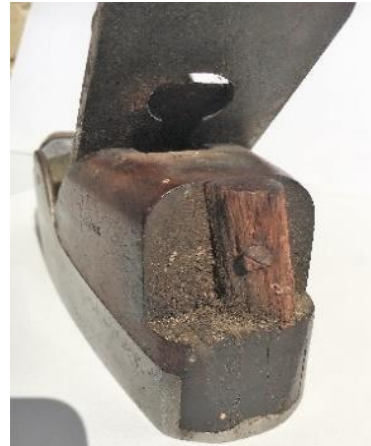
Figure 2. Major damage at rear of plane.
