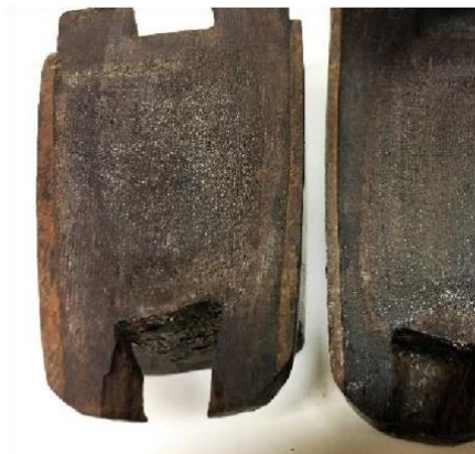
Figure 3: The rear infill made of two pieces of rosewood glued together
