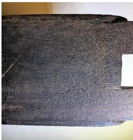
Figure 4: Showing side fillets glued to main part of rear infill
