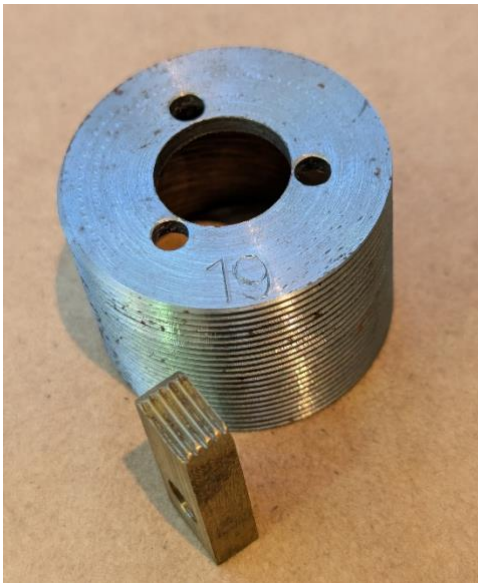
A 19tpi thread master made from its sub-master, together with its mating brass thread follower.
