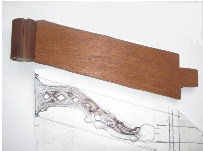
Sketch of a possible stretcher design with a blank stretcher and central boss for size guidance.
